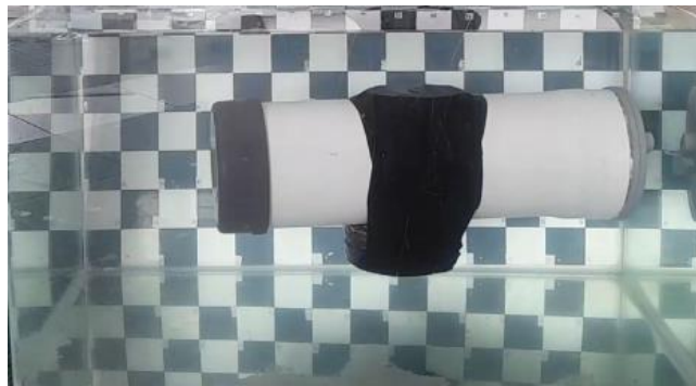
Figure 2. Experimental tank test for video-based displacement tracking: (a) schematic of the setup (checkerboard background, water level, and camera position), (b) submerged prototype in the test tank with the checkerboard reference
