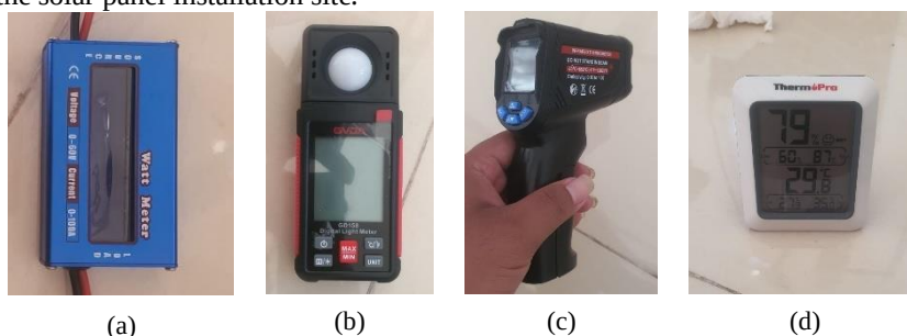
Figure 4. Measuring instruments: (a) digital wattmeter, (b) lux meter, (c) infrared thermometer, (d) thermometer
